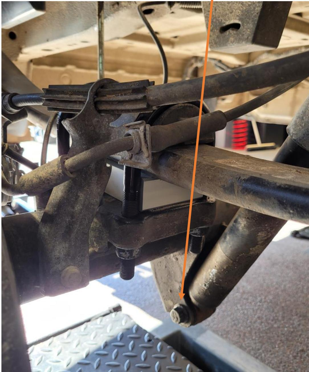
4. The dismantling of the rear axle series spring u-bolt is carried out according to the workshop manual!
